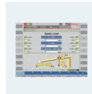
▲ System-specific special images are easily created and added to the standard interface with the integrated HMI editor.
